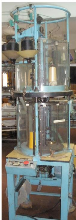
**Fig. 1.** Knitted circular binding knitting machine (the installation) with change the cylinder for the needles and the pushers
