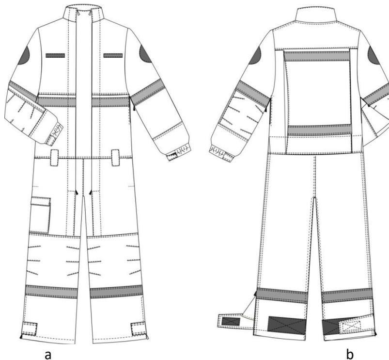
*Fig. 5. General view of the protective overalls for the elimination of the consequences of emergency situations in aviation, a – the front view, b – the rear view*
