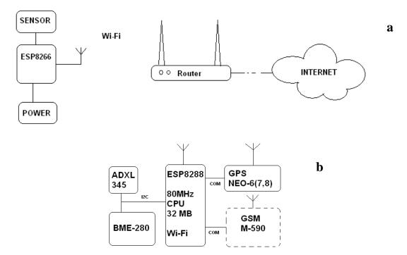
Figure 1 - The block diagram of the moving objects survey using a WiFi network (a) and GSM module (b)
