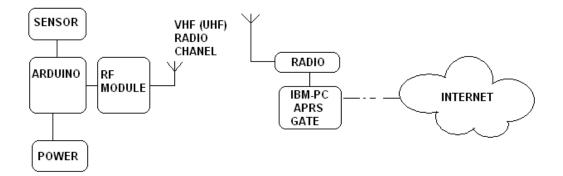
Figure 2 - Structural scheme of the system using the VHF radio network (range up to 100km)
