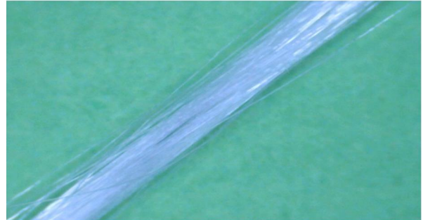
Figure 5 Diagram of polyamide filament yarn 29 tex consisting of 80 filaments, flat twist Kr=100 twists/meter, the nominal diameter d=2r=0.199 mm, the bending modulus B=2.6 \cdot 10^{-5} cN/mm 2
