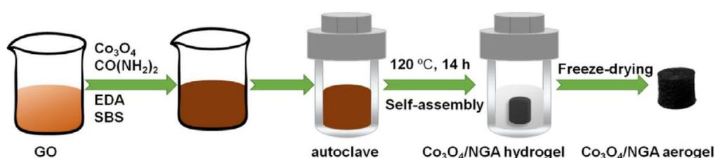
**Fig. 12. Schematic diagram for the synthesis of  $\text{Co}_3\text{O}_4/\text{NGA}$  catalyst[151]**
