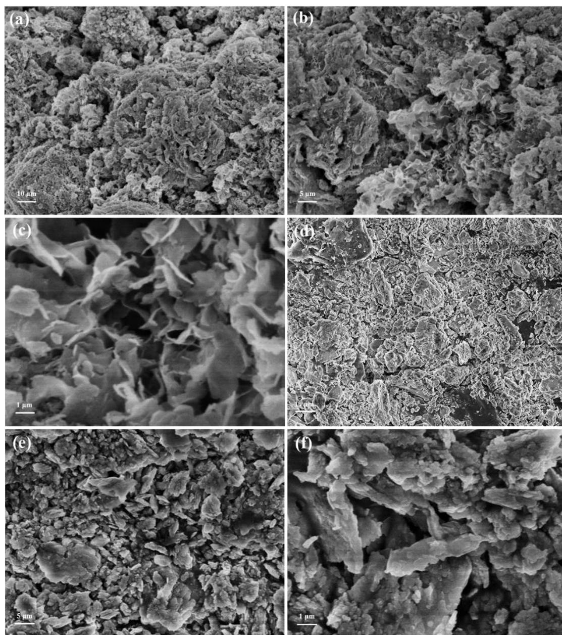
**Fig. 1.** SEM images of CoMn-LDH (a, b, c) and CoFe-LDH (d, e, f).
