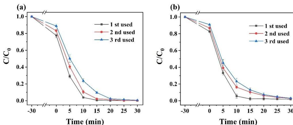
**Fig. 7.** Stability and reusability of CoMn-LDH (a) and CoFe-LDH (b) catalysts to activate PMS for 2, 4-DCP degradation. The diagram is the average value of the triplicate and the error bars represent SD. Reaction conditions:  $[2, 4\text{-DCP}]_0 = 20$  mg/L,  $[\text{PMS}]_0 = 0.2$  g/L,  $[\text{catalyst}]_0 = 0.2$  g/L,  $\text{pH}_0 = 6.5$  and  $T_0 = 25^\circ\text{C}$ .
