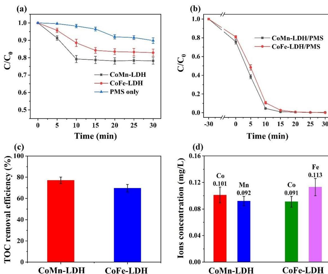
**Fig. 4.** Adsorption-desorption balance of CoMn-LDH and CoFe-LDH (a); catalytic degradation of 2, 4-DCP using different catalysts (b); TOC removal of 2, 4-DCP of CoMn LDH and CoFe-LDH (c); The concentration of cobalt ions, manganese ions
