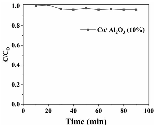
**Fig. 13.** Catalytic adsorption of TC of Co/Al<sub>2</sub>O<sub>3</sub> (10 %)
