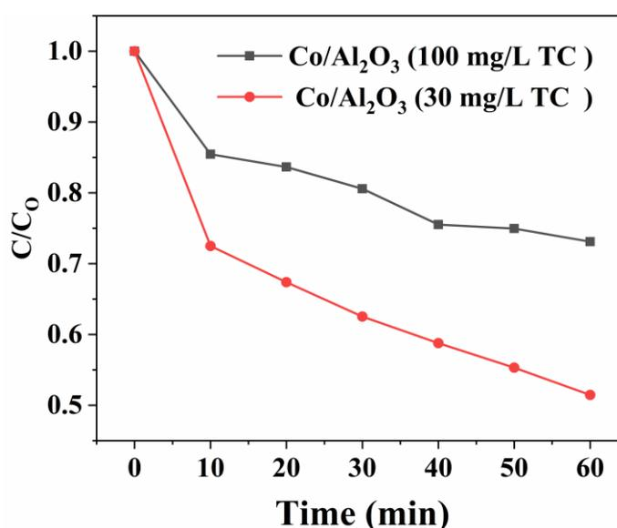
**Fig. 16.**Effect of TC concentration on TC degradation in Co/Al<sub>2</sub>O<sub>3</sub>/PMS system.
