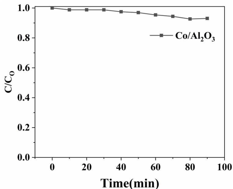
**Fig. 14.** Catalytic adsorption of TC of Co /Al<sub>2</sub>O<sub>3</sub> (10 %)
