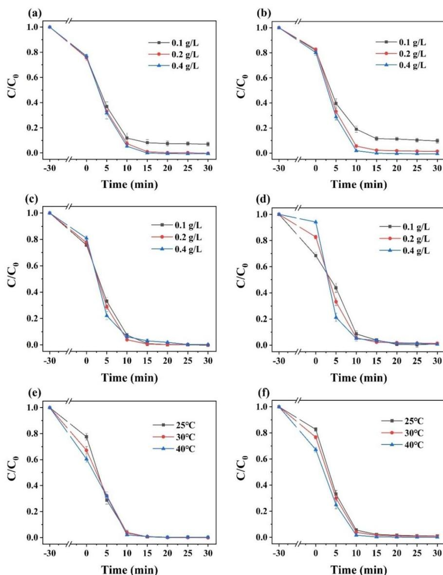
**Fig. 5.** Catalytic degradation of 2, 4-DCP under different conditions. PMS dosage
