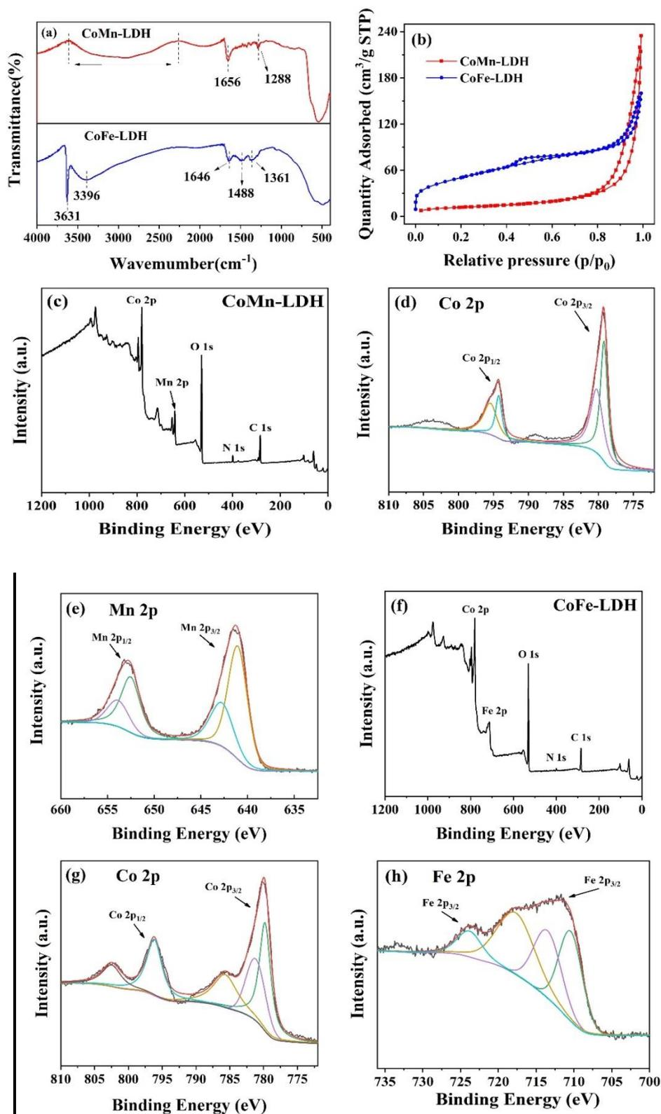
**Fig. 3.** FT-IR spectra (a) and N<sub>2</sub> adsorption-desorption isotherms (b) of CoMn-LDH and CoFe-LDH. XPS spectrum of CoMn-LDH (c) survey spectra: Co 2p (d) and Mn 2p (e); XPS spectrum of CoFe-LDH (f) survey spectra: Co 2p (g) and Fe 2p (h).
