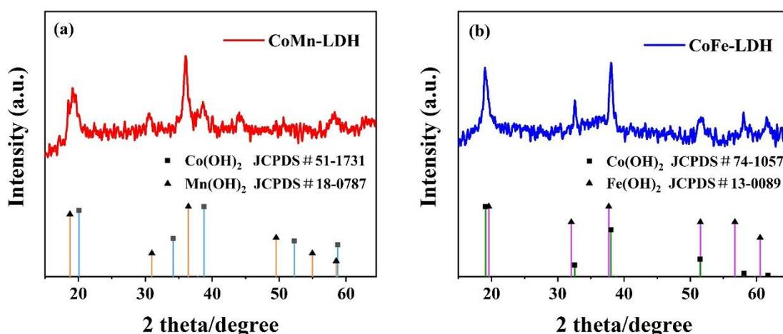
**Fig. 2.** XRD patterns of CoMn-LDH (a) and CoFe-LDH (b).
