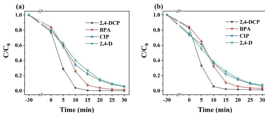
**Fig. 6.** The degradation of different pollutants by CoMn-LDH (a) and CoFe-LDH (b).
