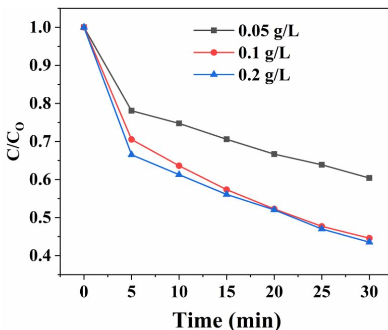
**Fig. 17.**Effect of PMS concentration on TC degradation in Co/Al<sub>2</sub>O<sub>3</sub>/PMS system
