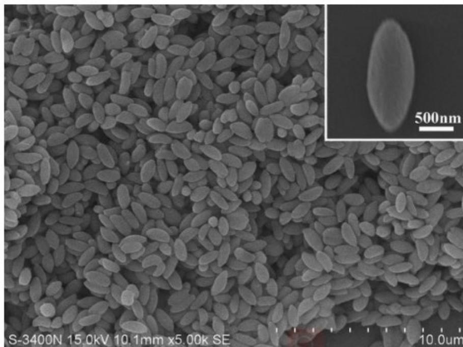
**Figure 1.11.** SEM image of the calcined ellipsoidal mesoporous silica. [67]
