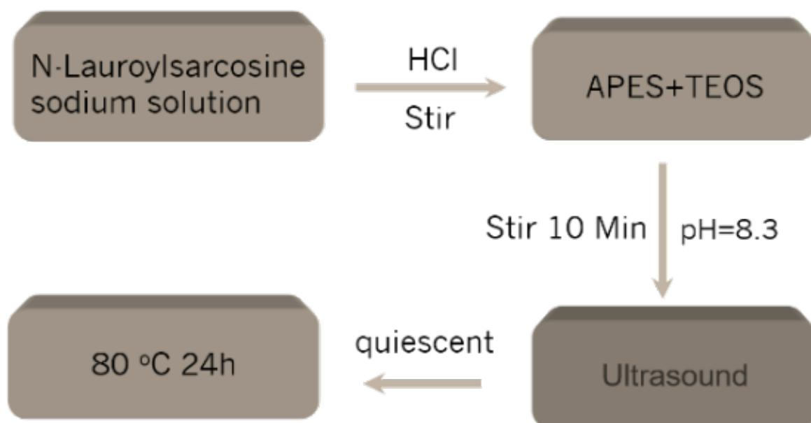
**Figure 2.1** synthetic procedure of mesoporous silica.
