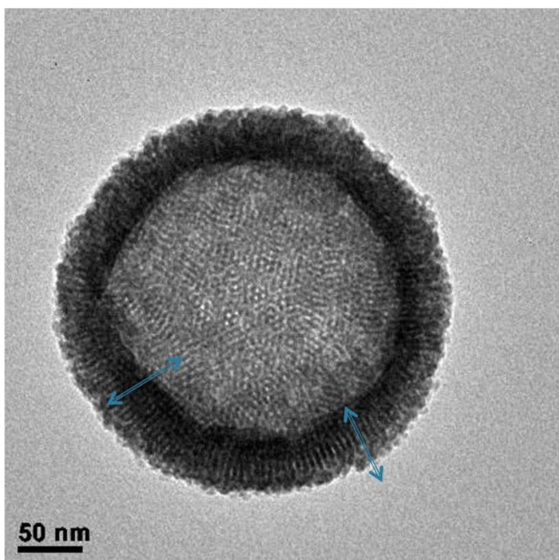
**Figure 2.2** TEM images of mesoporous silicon dioxide of MS-Hollow with a hollow structure.
