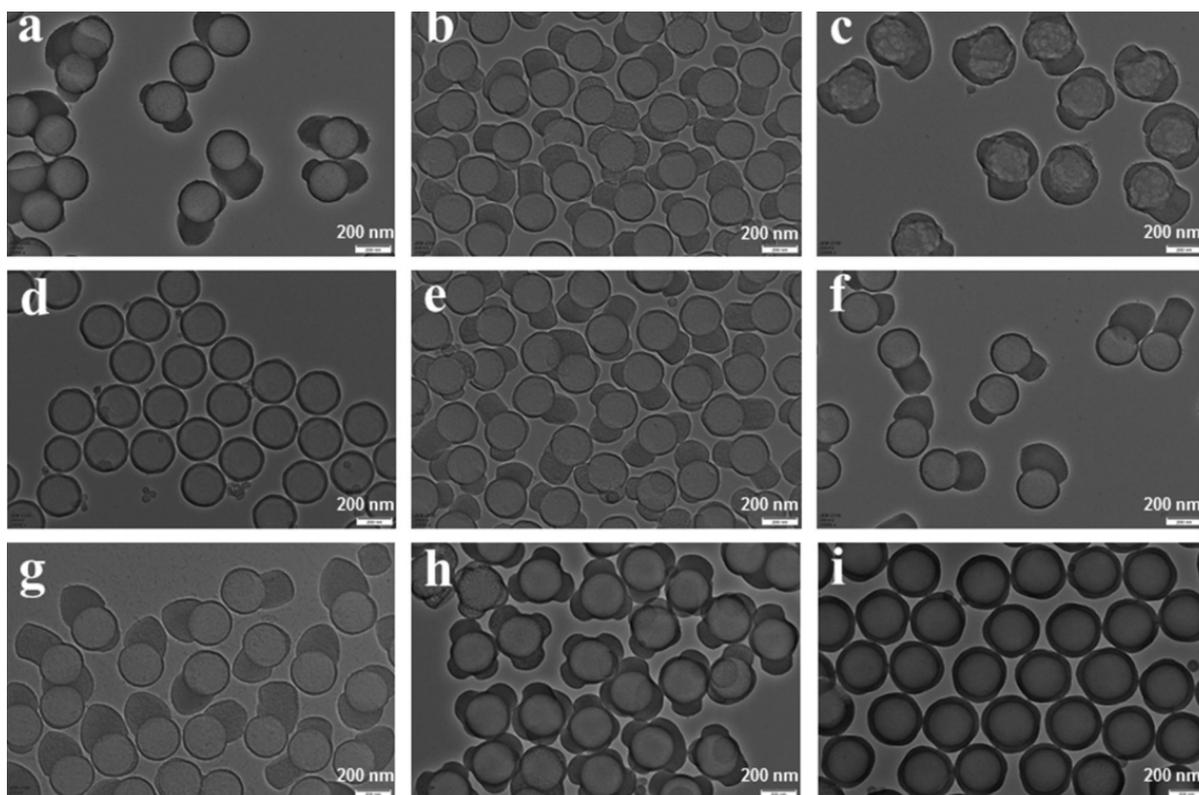
**Figure 1.10** Hollow mesoporous silica with different morphology and nano-structure [49].
