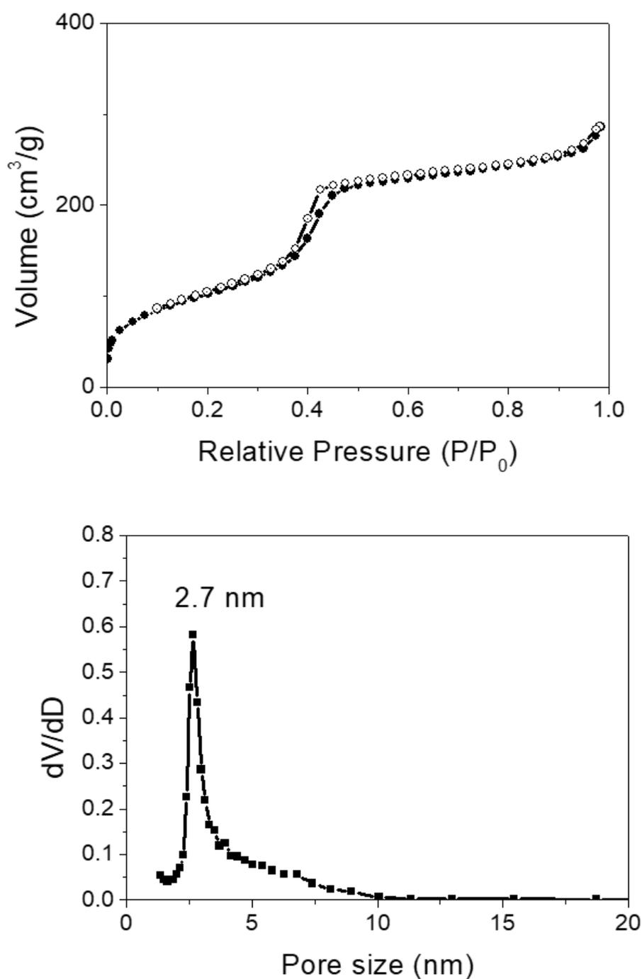
**Figure 2.5** (Up) Nitrogen adsorption-desorption isotherms and (Down) pore size distribution of MS-solid sample.
