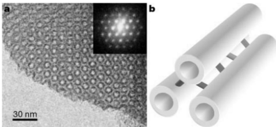
**Figure 1.2.** Ordered porous carbon prepared by template synthesis method using ordered mesoporous silica SBA-15. a) TEM image viewed along the direction of the ordered porous carbon. b) Schematic model for the carbon structure [15].
