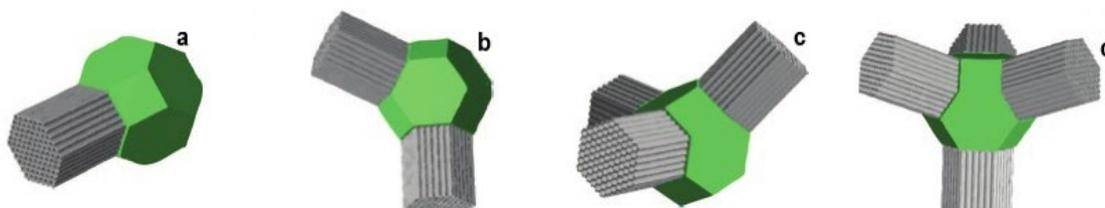
**Figure 1.12.** Schematic images of multicompart ment mesoporous silica nanomaterials with (a) one arm, (b) two arms, (c) three arms, (d) four arms [70].
