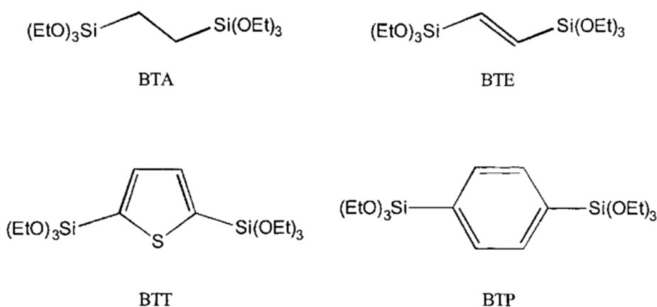
**Figure 1.6.** The molecular structure of alkoxysilane monomer bridged by an organic group [27].
