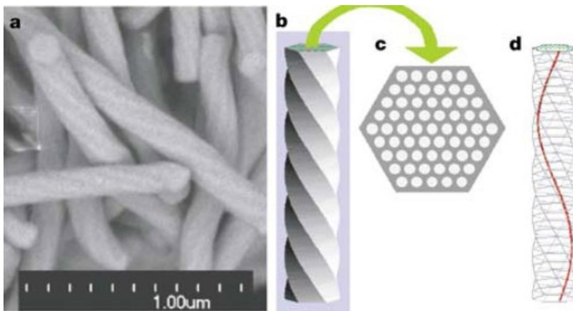
**Figure 1.3.** Chiral mesoporous silica [8].
