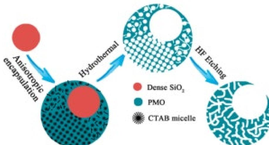
**Figure 1.14.** Preparing procedure for the asymmetric single-hole mesoporous nanocages [72]
