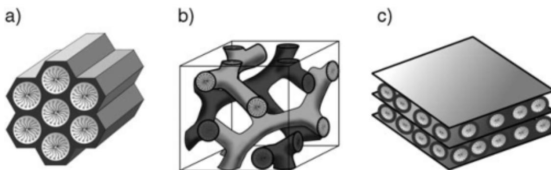
**Figure 1.1.** Structures of mesoporous M41S materials: a) MCM-41 b) MCM-48 and c) MCM-50. [2]
