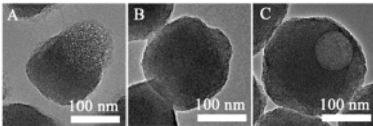
**Figure 1.13.** The TEM images demonstrating the morphology evolution of the eccentric nanocomposites [72].
