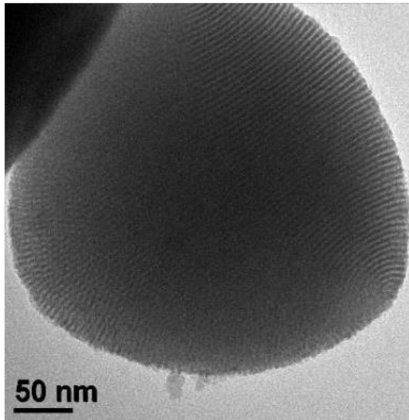
**Figure 2.3** TEM images of mesoporous silicon dioxide of MS-Solid sample.
