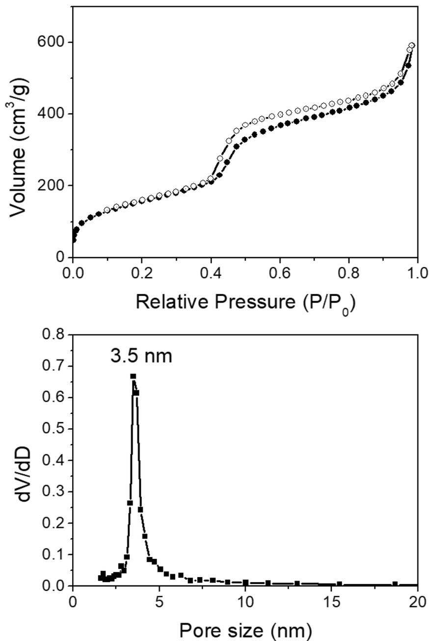
**Figure 2.4** (Up) Nitrogen adsorption-desorption isotherms and (Down) pore size distribution of MS-Hollow sample.
