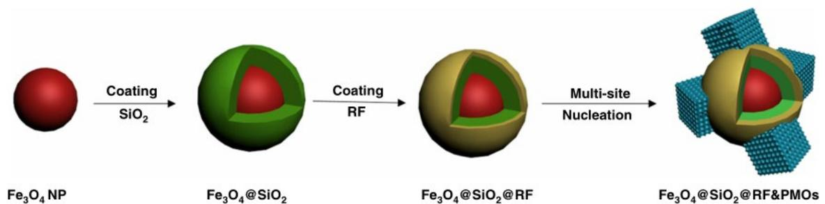
**Figure 1.15.** Illumination of complex mesoporous silica particles by adjusting the surface dynamics. [73]
