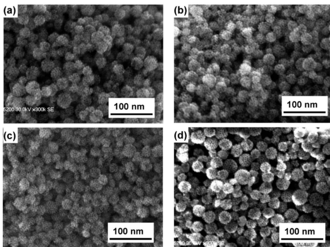
**Figure 1.8.** SEM images of the mesoporous silica nanospheres synthesized with different amounts of amino acid of arginine [44].
