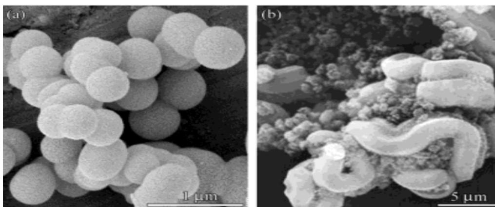
**Figure 1.7** (a) spherical MCM-41 by using the improved Stöber method and (b) regular MCM-41 by traditional method [31].
