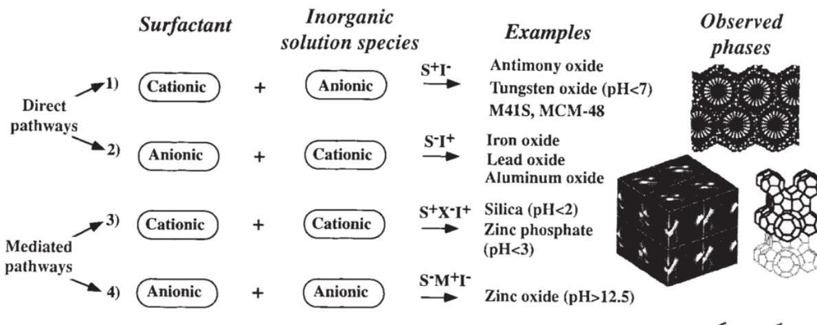
**Figure 1.5** cooperative self-assembly mechanism [20].
