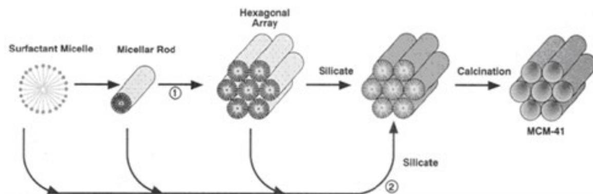
**Figure 1.4** ① Liquid crystal templating mechanism (LCT) and ② Synergistic mechanism (CFM) [11].
