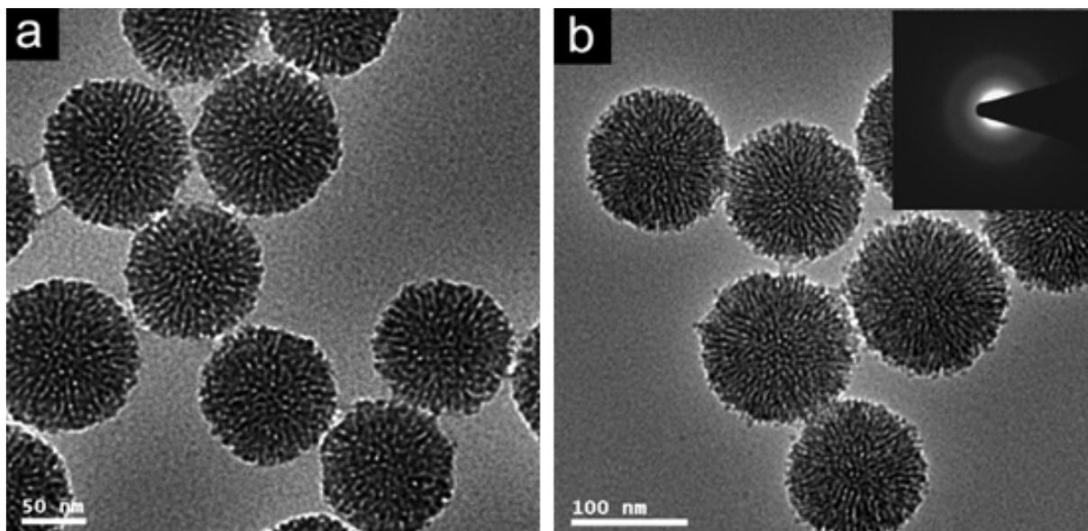
**Figure 1.9** Monodispersed mesoporous silica spheres with radially oriented mesopores templated from an anionic surfactant synthetic system. [47].
