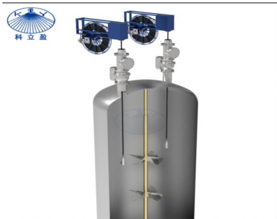
This equipment with heat preservation function, but also can withstand a certain pressure, because hydroxyethyl starch at room temperature dissolve slowly, at 60-70°C dissolve significantly faster, this equipment can play a certain purpose of optimization process.
