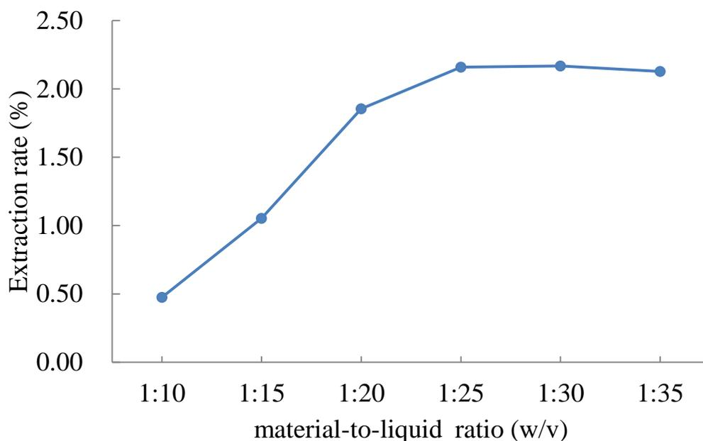
Figure 3-3 The effect of material-to-liquid ratio on the extraction rate of rose polyphenols
