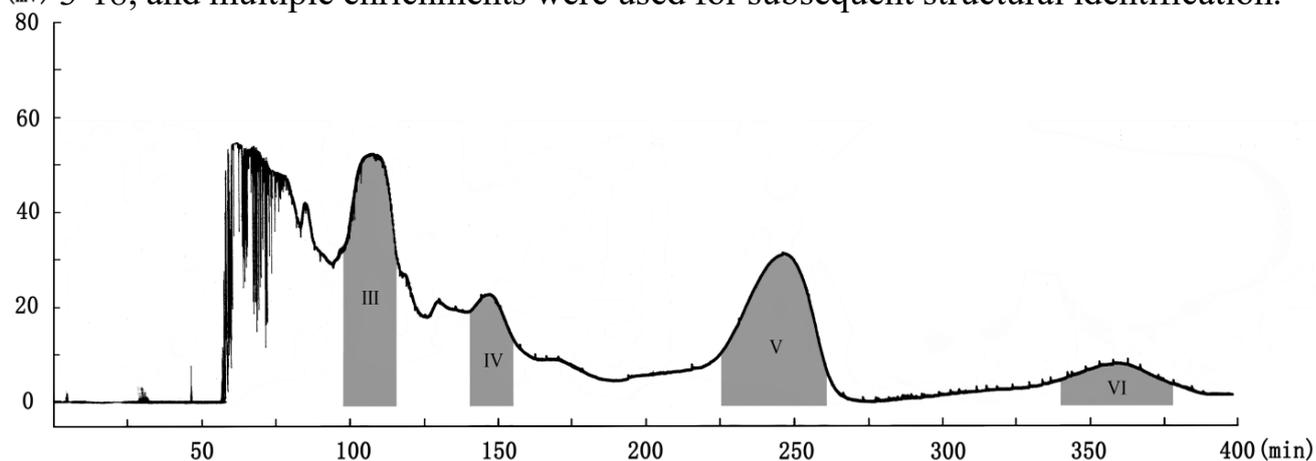
Figure 3-17 HSCCC separation diagram of recovered components of Dandelion. Solvent system: petroleum ether-ethyl acetate-acetonitrile-water (1:4:1:4, v/v/v/v); revolution speed: 800 rpm; flow rate: 2.0 mL/min; sample size: 400 mg; UV detection wavelength: 280 nm.
