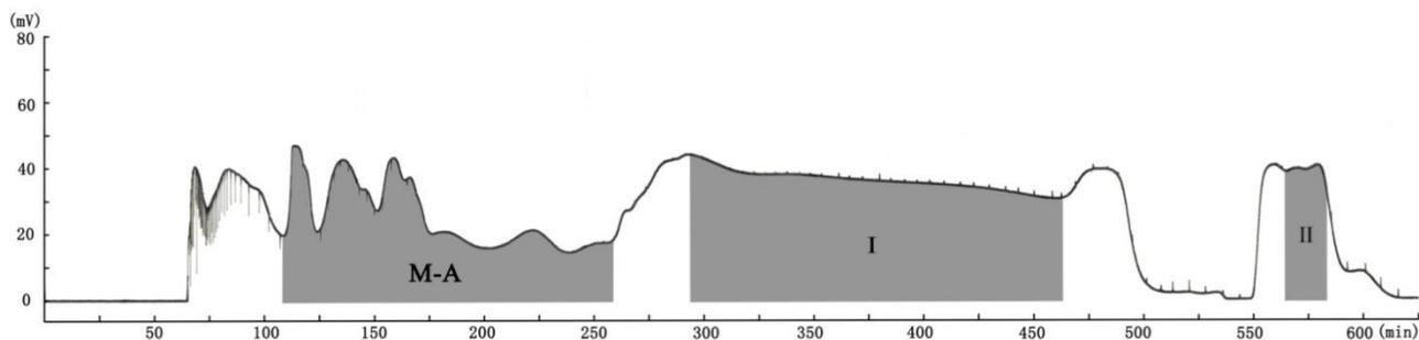
Figure 3-15 pH-ZRCCC separation diagram of crude extract of Dandelion. Solvent system: ethyl acetate-n-butanol-water (4:1:5, v/v/v); TFA (10mM) in upper organic phase, ammonia (10mM) in lower aqueous phase; revolution speed: 800 rpm; flow-rate: 2.0mL/min; sample size: 1.6g; UV detection wavelength: 280nm.
