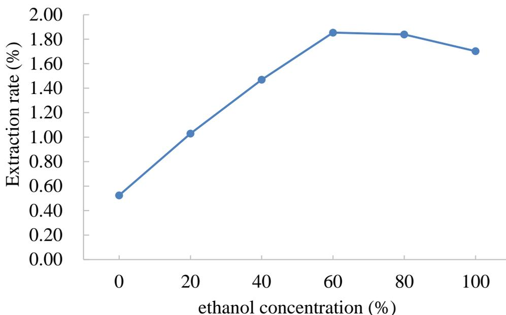
Figure 3-2 The effect of ethanol concentration on the extraction rate of rose polyphenols
