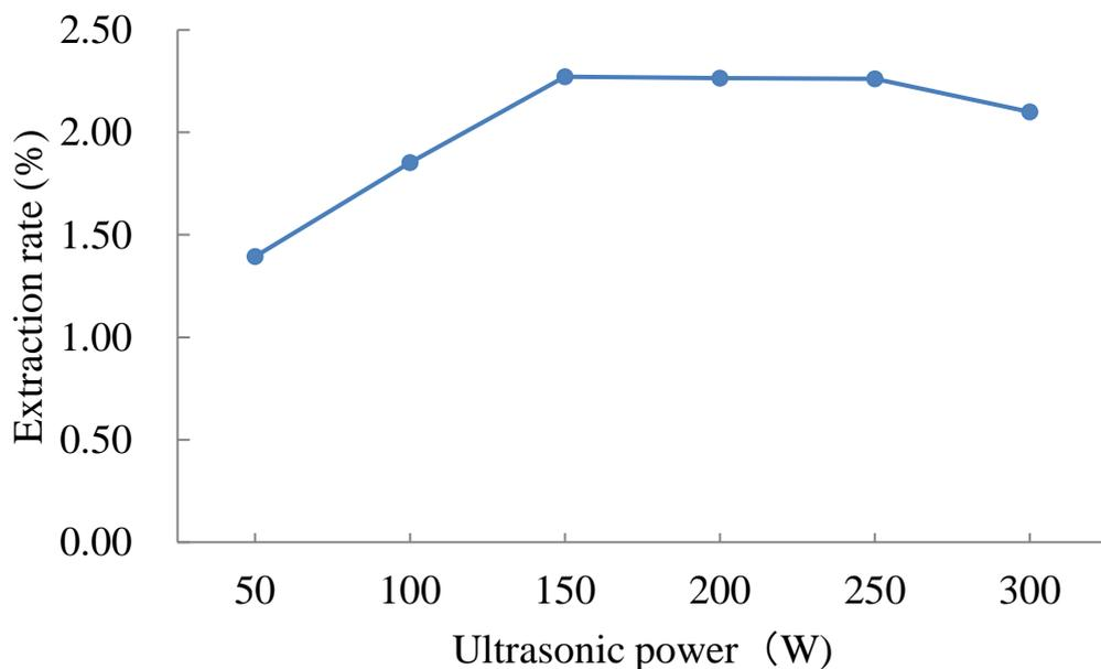
Figure 3-5 The effect of ultrasonic power on the extraction rate of rose polyphenols
