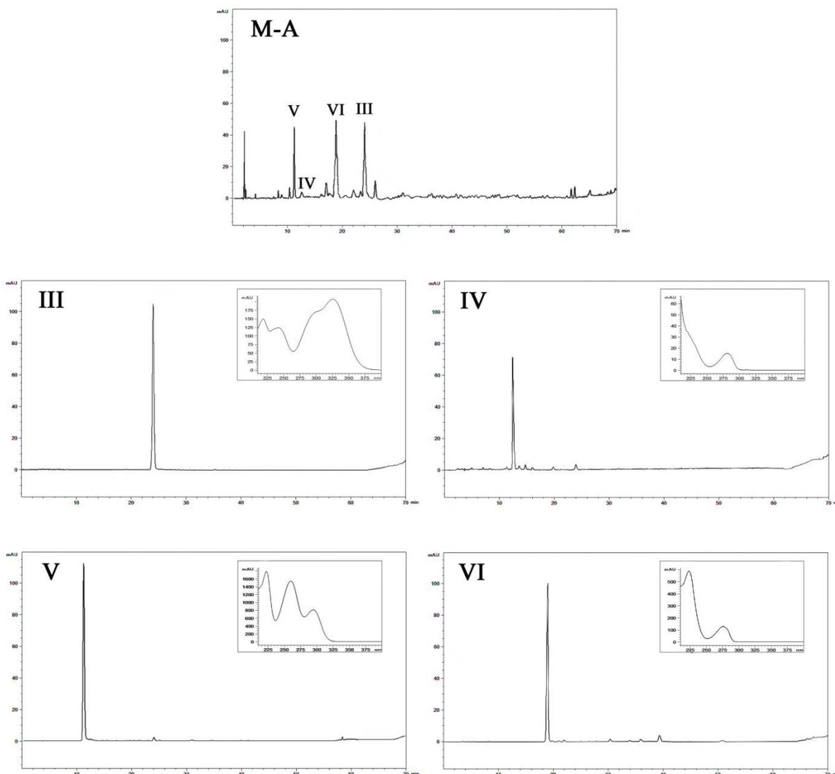
Figure 3-18 HPLC chromatograms of Mixture M-A and components separated by HSCCC. (M-A) Mixture M-A; (III) 1-O-caffeoylglycerol; (IV) 3,4-dihydroxyphenylacetic acid; (V) protocatechin; (VI) *p*-hydroxyphenylacetic acid.
