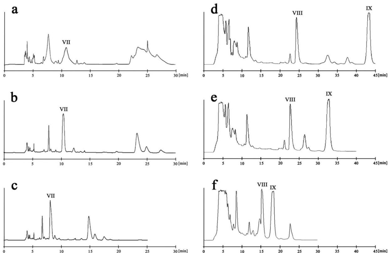
Figure 3-19 Effects of composition of mobile phase on separation. (a) Sample T-W, methanol-water (28:72, v/v); (b) Sample T-W, methanol-0.1% formic acid water (28:72, v/v); (c) Sample T-W, methanol-0.1% formic acid water (32:68, v/v); (d) Sample T-60, methanol-water (55:45, v/v); (e) Sample T-60, methanol-water (58:43, v/v); (f) Sample T-60, methanol-water (60:40, v/v)
