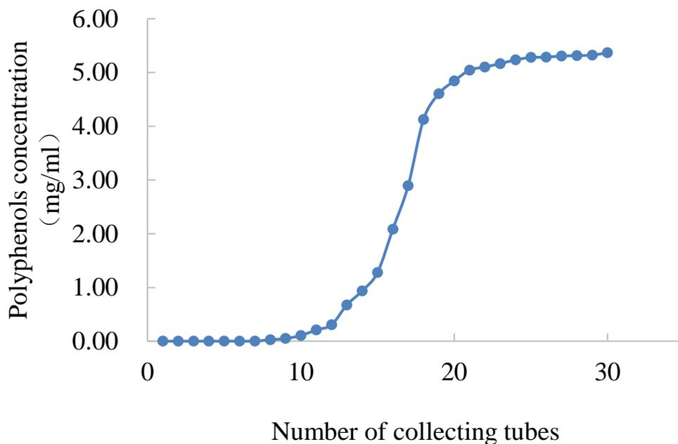
Figure 3-7 The leakage curve of rose polyphenols
