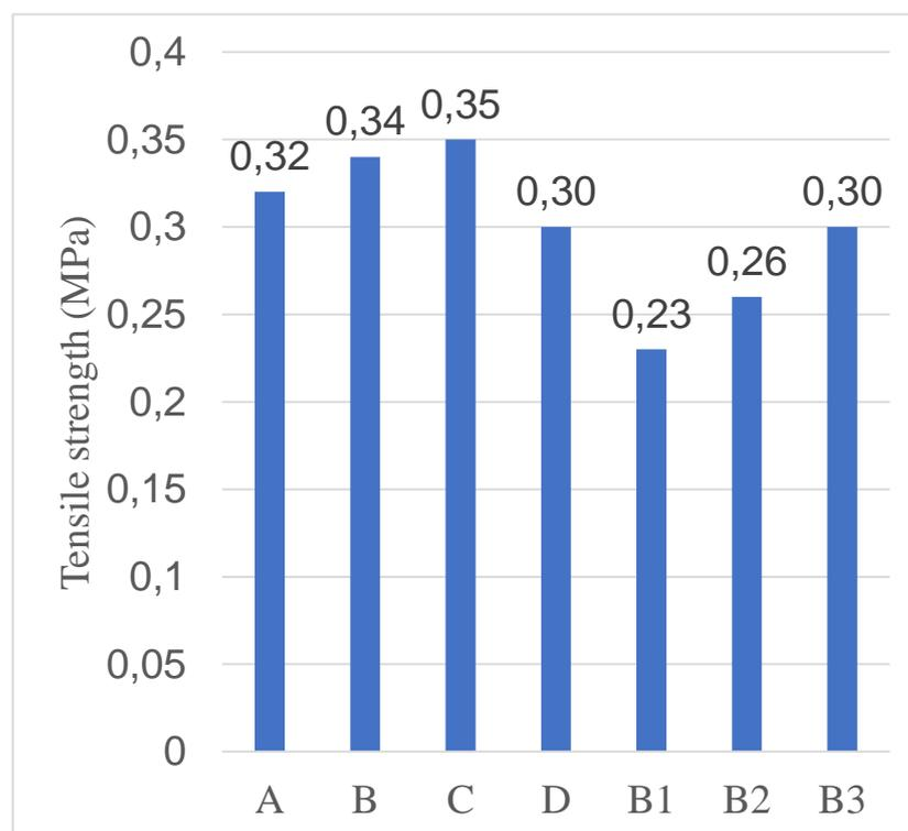
Figure 2.13 – Tensile strength of PVA film
