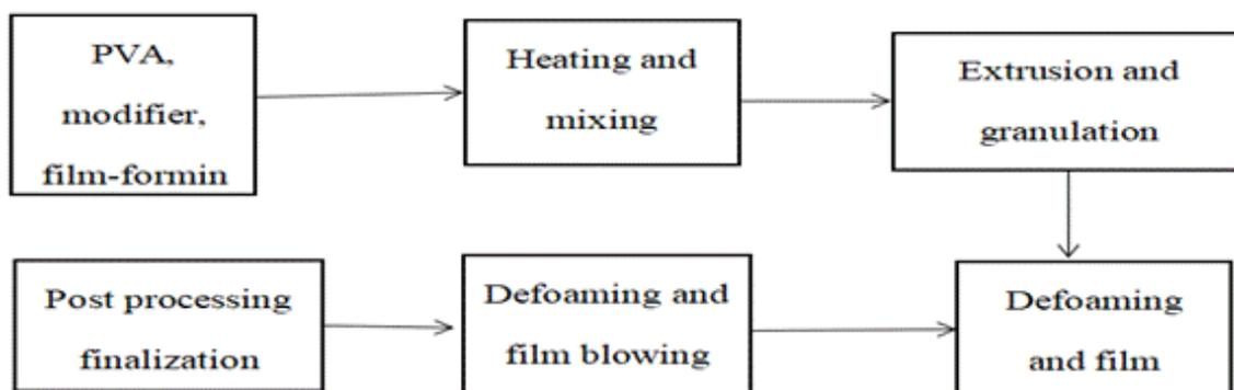
Figure 1.9 – Flow chart of dry extrusion blow moulding method
