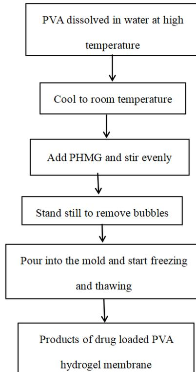
Figure 3.5 – Process flow chart of preparation of PVA hydrogel film
