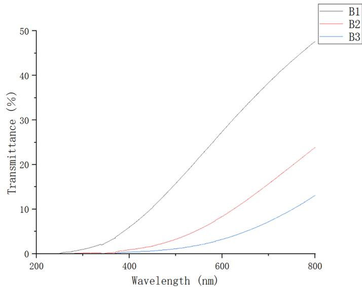
Figure 2.8 – Transmittance of PVA film with different freeze-thaw times and the same drug loading concentration
