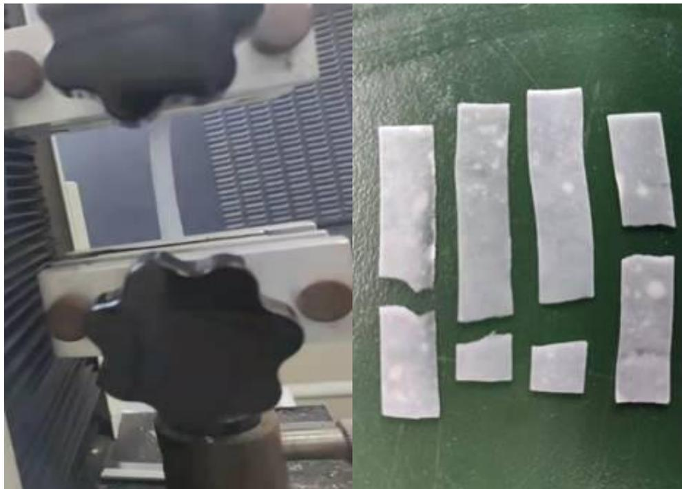
Figure 2.11 – PVA membrane mechanical test and after test
