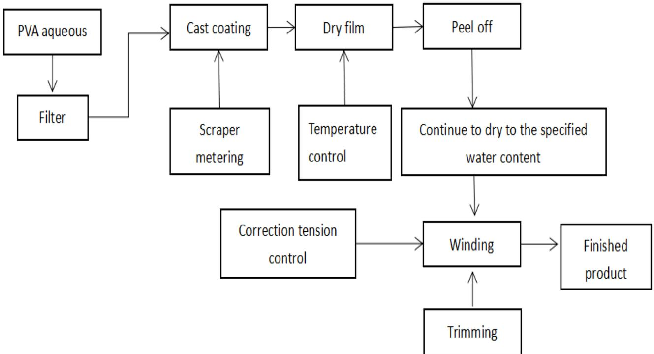
Figure 1.7 – Flow chart of casting method
