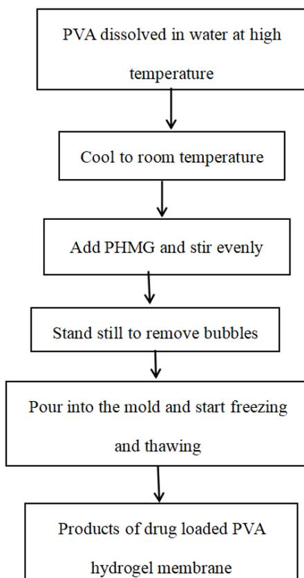
Figure 2.1 – Process flow chart for preparation of drug-loaded PVA hydrogel membrane
