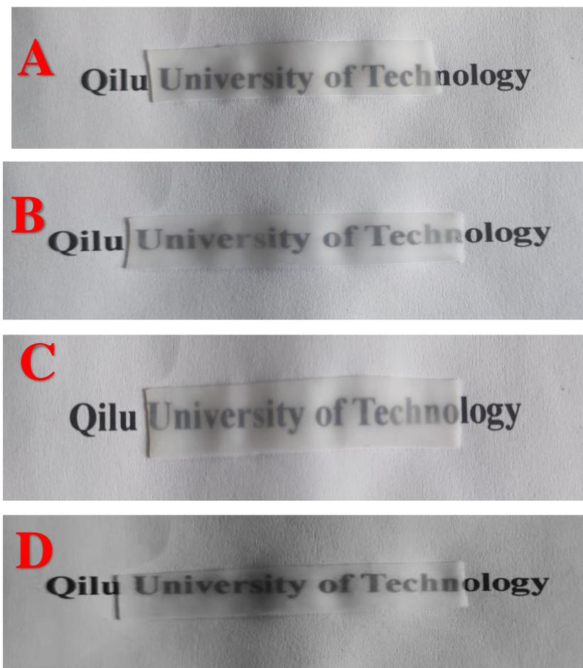
Figure 2.5 – The appearance of PVA membrane with the same freeze-thaw times and different drug loading concentrations
