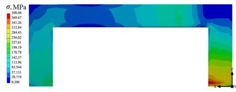
**Figure 4.** The distribution of the fields of stresses  $\sigma$  according to Mises in the flexible plate for cam at the loading  $\overline{F}_{lif}$  =14.03 N and the width of the console beam of the plate B = 3.17 mm.
