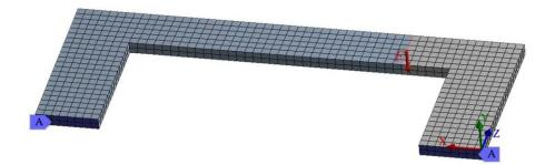
Figure 1. The model of the flexible plate for the cam according to the finite element method: F – force; A – areas of the hardcover of the plate.
