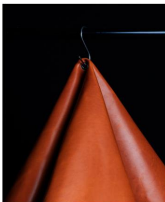
Figure 3. Leather tanned with Pinus pinaster bark modified extract
