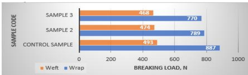
Fig. 1. Comparison of the breaking load of tested samples, N
