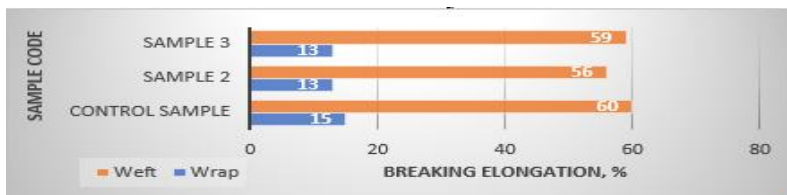
Fig. 2. Comparison of the breaking elongation of tested samples, %
