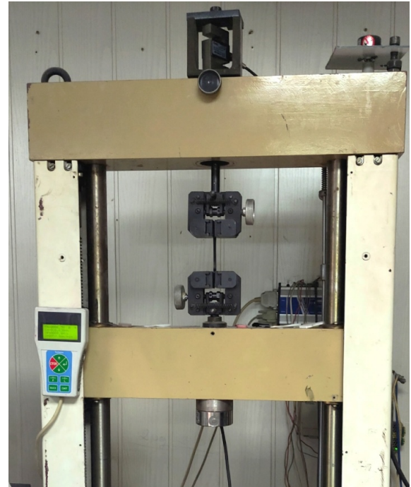
Fig. 5. Modernized rupture machine 2167 P-50
