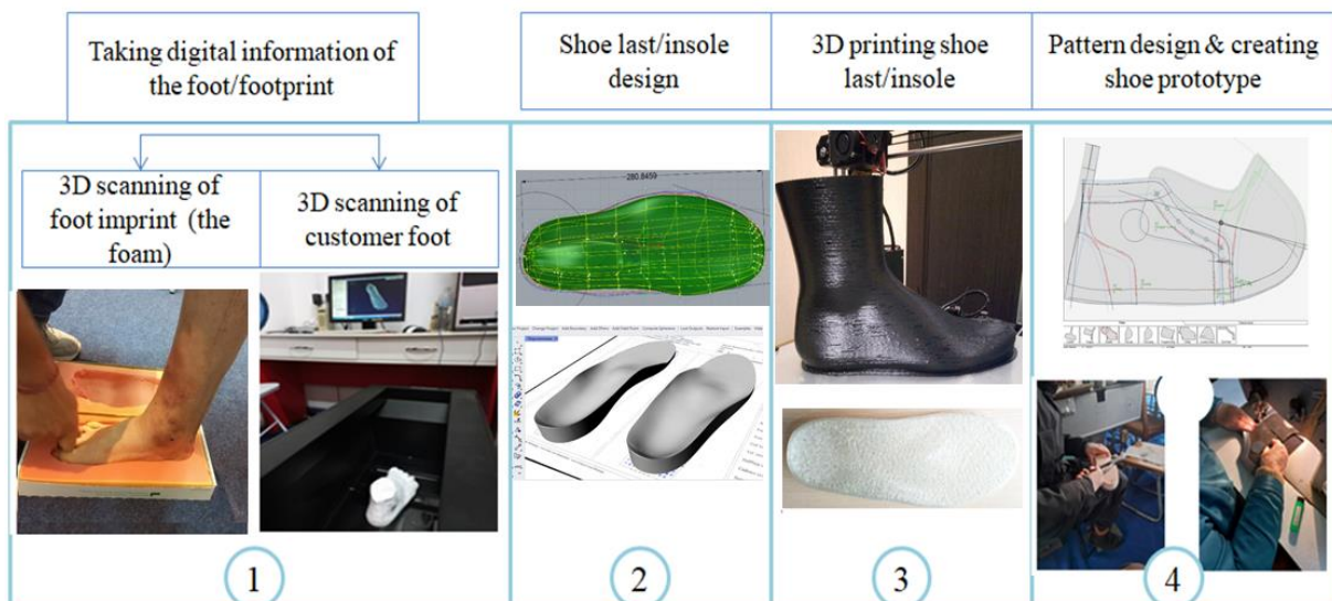
Figure 8: The main stages of process of creating the personal orthopedic footwear.
