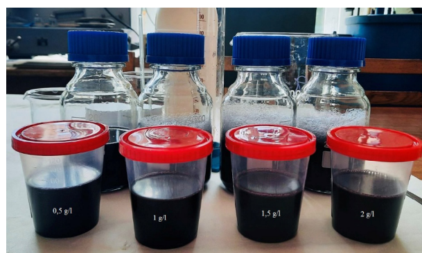
Fig. 3. Dispersions of Setaprs Black CE-RN dye with nonionic surfactant of different concentrations
