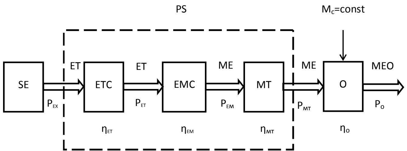
Figure 1 – functional energy structural scheme of unmanageable electric drives.
