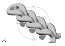
Figure 1 3D geometric model of a plainknitted structure
