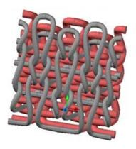
Figure 2 3D geometric model of a weft double-layer knit with tuck connection flayers
