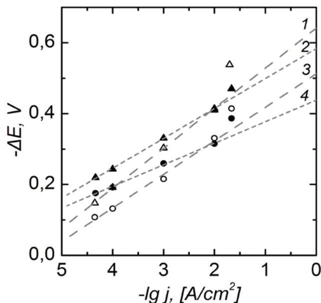
**Fig. 2.** Semilogarithmic dependencies of hydrogen evaluation overvoltage on current density in 1M NaOH at the cathode materials ( $t = 25\text{ }^{\circ}\text{C}$ ): 1 – steel 45; 2 – steel 45 coated by nickel; 3 - 12Cr1MoV steel; 4 – steel 45 coated by vanadium-doped nickel
